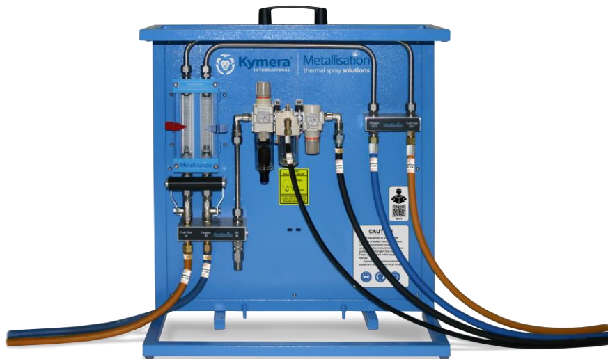
Supplies from regulators to flowmeters
