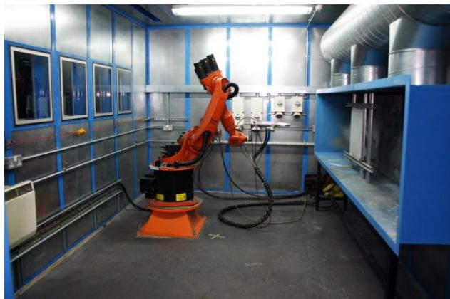
The company has also invested in a demonstration and testing facility, incorporating a 6-axis Kuka robot, spray booth and extraction unit. This will enable Metallisation to facilitate more Research and Development projects and develop tailor made processes with its customers. It also allows the company to demonstrate the whole product range more easily and enhance its customer solution delivery.
