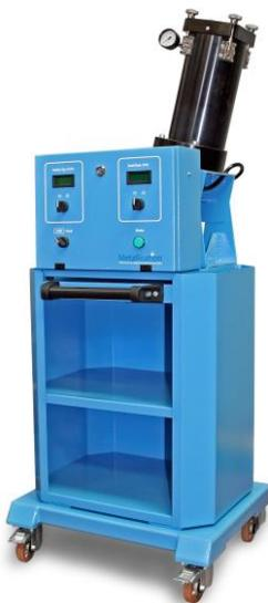
The 2007MF-PF-HC powder feeder is a positive displacement feeder which uses an offset disc that rotates and collects powder in small holes. At a certain point powder is blown from the holes into the powder feed line where the Argon gas carries the powder through the powder feed hose to the required point of exit.
