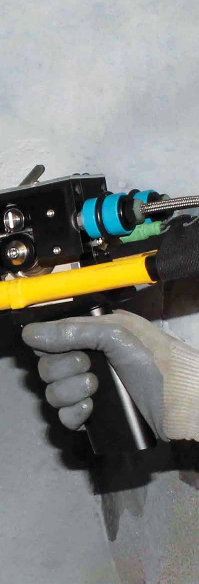
Thermal spraying, also commonly known as metal spraying, is a surface engineering/coating process whereby a wide variety of metals, ceramics and polymers can be sprayed onto the surface of another material. The range of materials that can be sprayed is almost limitless - if the material can be heated to its melting point without boiling away, then it can be thermally sprayed.
