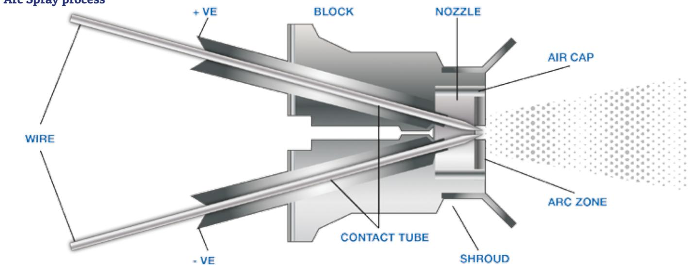
charged, one positive and one negative. The wires are forced together and form an electric arc, melting the wire. Compressed air, passing through a nozzle, atomises the molten metal and sprays it onto the work piece. There are three methods of wire feeding; push, pull and push/pull. The higher the current rating of the system, e.g. 350A, 700A etc., the higher the spray rate.
