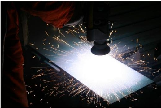
28E ARCTEC is applied using the Metallisation arcspray process with the ARC 140 system. In the arcspray process the raw material, in the form of a pair of metallic wires, is melted by an electric arc. This molten material is atomised by a cone of compressed air and propelled towards the work piece. Upon contact, the particles flatten onto the surface, freeze and mechanically bond,
