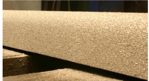
Untreated steel surfaces can become very slippery, especially in wet conditions, and are prone to corrosion. To ensure safe walking and industrial operating conditions, vital to personal safety and corporate productivity, 28E ARCTEC coating provides a durable non-slip anti corrosion coating.
