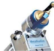
Metal spraying involves the projection of small molten particles onto a blast prepared surface. Upon contact, the particles flatten onto the surface, freeze and mechanically bond, firstly onto the blasted substrate and then onto each other, as the coating thickness is increased. To create the molten particles, a heat source, a spray material and an atomisation/projection method are required.
