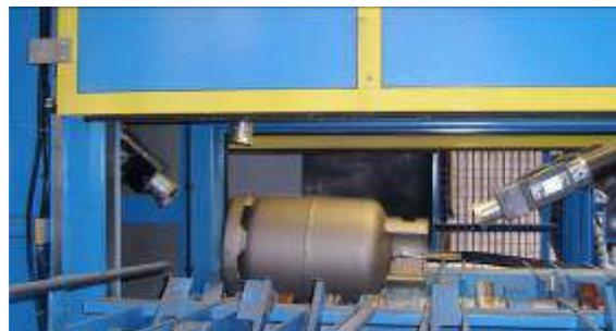
The machine is also supplied with dust extraction and dry filtration equipment, to ensure there is no contamination of the coating and to provide a safe working environment.
