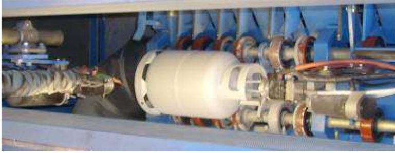
Each bottle is coated with an average of 60 microns of zinc. The base of the bottles is coated with a slightly thicker coating to provide greater protection in an area normally subjected to
