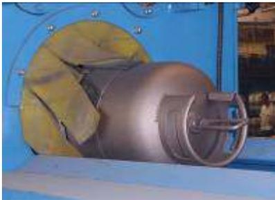
Vitkovice Milmet make the bottles by first pressing the parts which are then welded together with the fixtures, before pressure testing them prior to applying a surface coating. The surface of the bottles needs to be prepared to ensure an adequate profile is created for metal spray adhesion. This is done by grit blasting the bottles in an automatic blasting machine, which produces a blast cleanliness of SA 2.5. Once the surface has been prepared, the metal spraying can begin.
