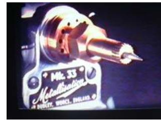
In the Metallisation Flame spray process, the raw material in the form of a single wire, cord or powder, is melted in an oxygen-fuel gas flame. This molten material is atomised by a cone of compressed air and propelled towards the work piece.
