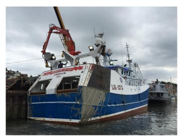
thermal sprayed zinc base layer clearly remains and continues to protect the hull from rust.
