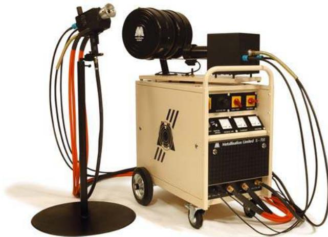
Constant Geometry (CG) head, which ensures a smooth and consistent spray quality. In addition, the all new 700Amp energiser is designed with a harsh environment in mind, with all control electronics sealed from dust intrusion. All these factors combined, result in unrivalled spray rates, superior reliability and excellent time and cost savings. The system can be packaged for workshop and site applications giving clients optimum ease of use in a range of situations.
