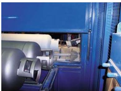
With the bottles still in their horizontal position following the grit blast process, they are transferred from the blast room to the spray booth. Zinc is applied by three Metallisation Arc 528 systems: Two Arc 528/S250 amp systems apply a coating of 75 microns to the base of the cylinder and 50 microns to the top, while an Arc 528/S450 system traverses along the bottle and applies a 50 micron coating to the sides.
