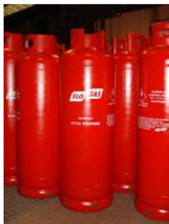
The bottles then exit the spray booth and are returned upright, base down and carried through to the wet paint section via conveyors. Painting of the bottles is an automated process, where two-pack epoxy paint, in Flogas colours, is applied before oven drying. Once dry the Flogas logo, safety data, new tare weight and test dates are all applied by screen printing and the application of a metal data disc. The bottles are then purged and re-valved and despatched to on or off site filling plants.
