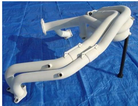
The Woof plasma ceramic coatings can reduce surface temperatures by up to 160°C and can withstand temperatures of up to 1400°C. This compares with typical standard ceramic containing paint, which may only reduce surface temperatures by up to 9%.
