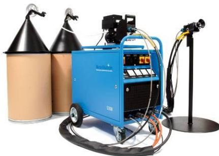
‘Synchrodrive’, which reliably and positively drives the wire at the dispenser and the pistol, allowing the pistol to be up to 20m from the wire. The flexible drive system means that there is no motor in the pistol, resulting in a lightweight, manoeuvrable pistol, increasing the flexibility of the system and reducing operator fatigue.
