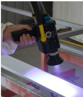
In the metal spraying process surface preparation is very important to the success of the final coating. All of the surfaces are therefore prepared by grit blasting with steel grit to SA 2.5, which ensures the surface area is ready to accept the metal sprayed particles. Electro Metal Depositors aims for around 70 - 100 microns of zinc spray and between 70 – 100 microns of powder coat, which gives a total of 140 – 200 microns of protective coating on all projects.
