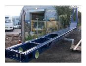
The L&RS will be consistently exposed to harsh seawater environments and therefore needs to be protected from corrosion. Supacat specified metal spraying with zinc as the most effective corrosion protection and commissioned Perryfields to complete the project. The front and rear chassis' have been specified by Supacat
