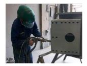
The deflected flame spray extension was launched in July 2010 and Perryfields was one of the first companies to purchase the new equipment. Perryfields Limited, painting and finishing specialists, based in Dorset, added the flame spray extension to its existing range of metal spraying equipment because of its ability to apply a
