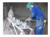
process, or suspended in organic compounds, ensuring maximum cathodic corrosion protection, similar to galvanising.
