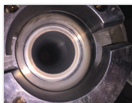
Battery Insert After Coating with CASL UHD ID HVOF™
