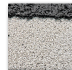
HaloJet™ WCCoCr Coating in a 3" ID
