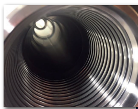
Cleaned HaloJet™ coated shock jar after 263 hours in service
